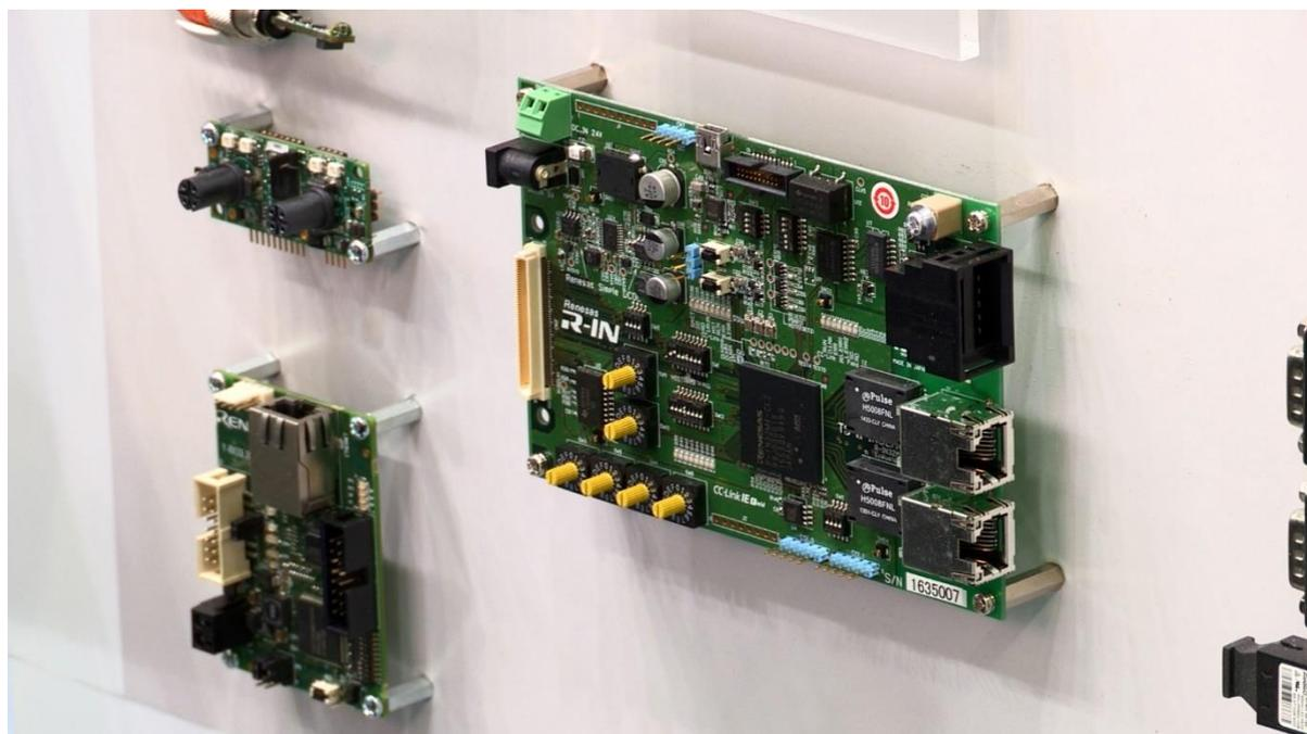
The R-IN32M4-CL2 can now support CC-Link IE network connectivity with minimal external components, leading to simplified and cost-effective system designs.
